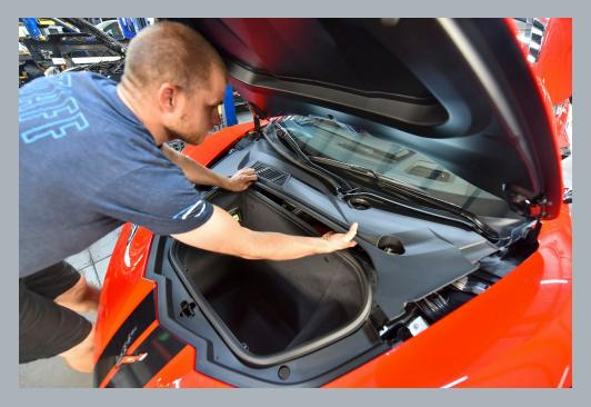
Once you've removed the trim pieces go ahead and take your 10mm socket or wrench and disconnect the negative terminal from the battery.
