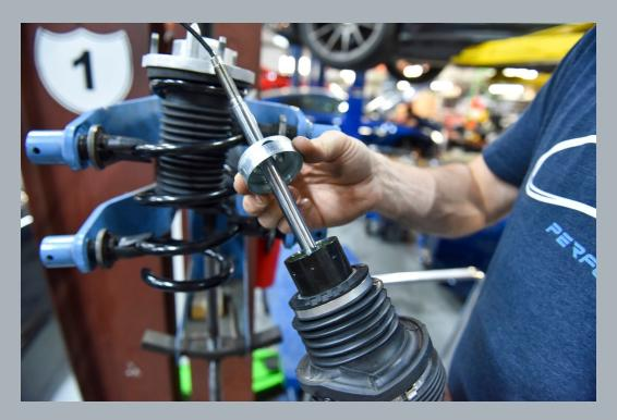
Sliding the front lift assembly off of the strut will give you access to the silver factory front lift collar. This silver collar can also be removed by simply sliding it off the top of the strut. Now you're ready to install your new Cicio Performance components!
