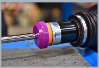
Slide your freshly cut bump stop onto the strut with the purple cap pointing towards the top.
