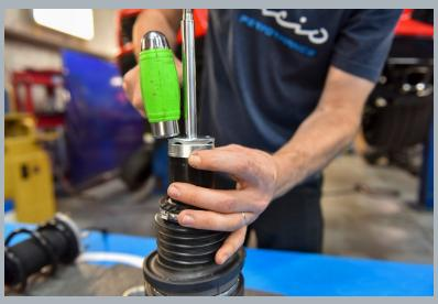
Mark the suspension bump stop (purple capped foam) at the line seen in the image below. You'll be cutting the bump stop at this line and discarding the lower piece of the bump stop marked with the Chevy part number.
