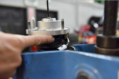
Install the nut back onto the top of the strut and tighten it to  $^{\sim}50-60$  ft lbs.
