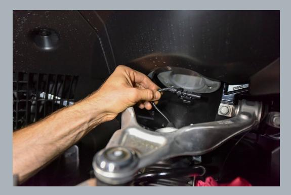
If you're starting with the driver side turning the rotor / hub assembly slightly to the right will help give you the additional clearance needed to remove the strut body. When tackling the passenger side turning the rotor / hub assembly slightly to the left will give you the additional clearance needed to remove the strut body.
