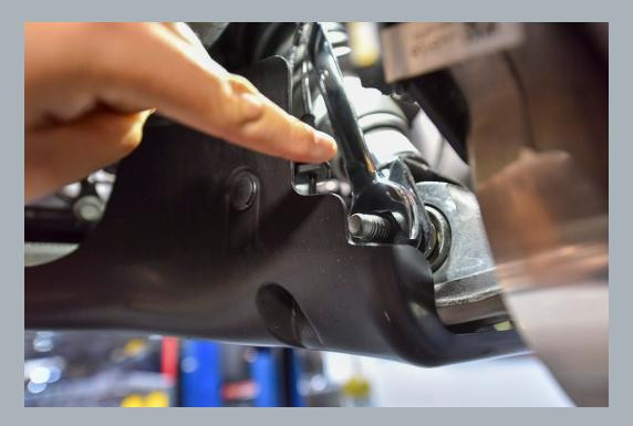
You may find the pushing downwards on the brake rotor / hub assembly will help you remove the 21mm bolt securing the strut to the lower control arm.
