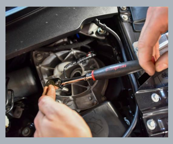
If your vehicle is equipped with Magnetic Ride Control (MRC) like our's is you'll have to pull the red tab back on the MRC plug in order to disconnect the wire.
